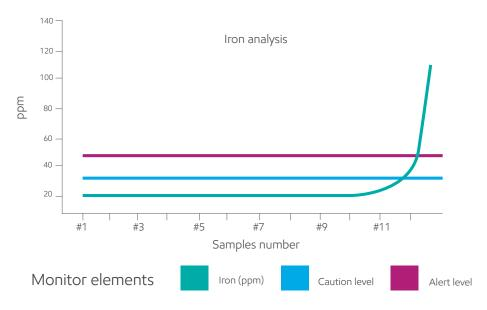
The caution and alert bars represent levels. The geometric rate of wear increase represents the trend. Both the trend and the level indicate that this is a severe problem.
